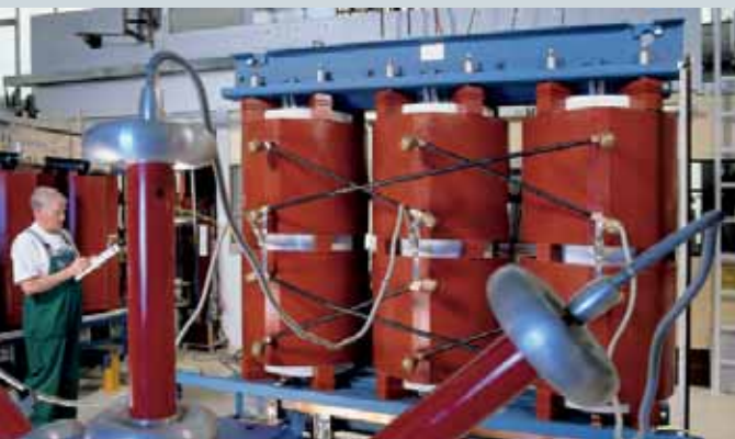
Figure 1: GEAFOl cast-resin transformer in the test bay at the Siemens transformer plant in Kirchheim/Teck: If GEAFOl cast-resin transformers are involved by an external fire, they don't significantly affect the course of the fire thanks to their low fire load. Nor do their coils ignite from short-circuit arcs caused by intrinsic flaws. Moreover, no toxic components are produced, other than the type of flue gases common to fires.
