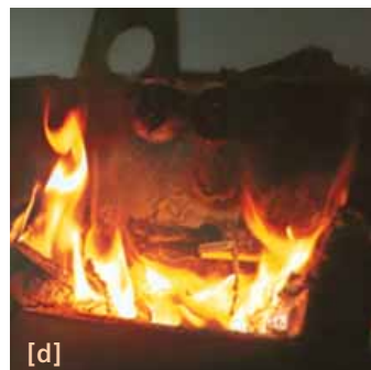
Figure 7: Combustion sequence during exposure by the external propane gas fire. a) After six minutes b) After eight minutes c) After 20 minutes d) After 33 minutes
