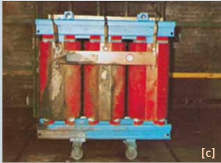
Figure 4: GEAFOLE cast-resin transformer in the short circuit arc test:
