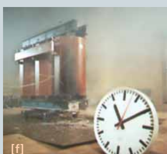
Figure 6: Combustion sequence during exposure to flames of the external wood fire: The outer surface of the HV winding was ignited only in the immediate area of exposure to the external fire, and hardly any fire spread to the adjacent leg.
