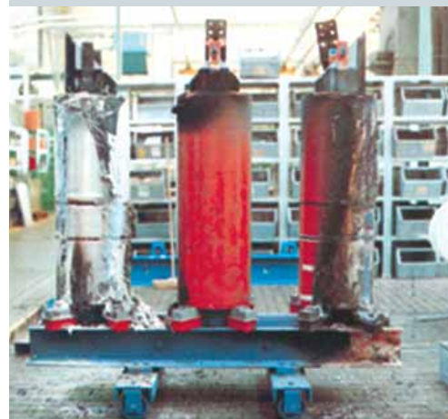
Figure 9: LV windings after the fire behavior test: Surfaces exposed directly to the flames were severely affected, while adjacent portions of the insulating material remained largely undamaged. Even in the leakage channel the fire was did not spread horizontally – despite the extremely abundant input of oxygen.
