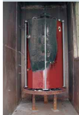
Figure 3 a + b: Very good resistance to direct flame action was certified: 1,500-kVA GEAFOL cast-resin transformer under test at the CESI Test Institute in July 2005 before (above) and after (below) testing to verify compliance with IEC 600076 fire category F1.
